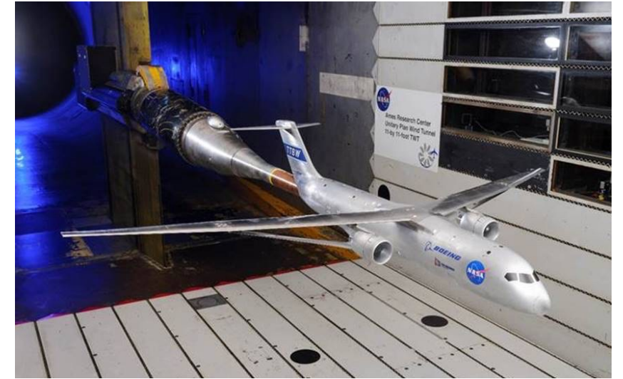
NASA/Boeing 4.5% Scale Transonic Performance Test NASA Ames Research Center Primary Plane Wind Tunnel (14 by 19-foot TWT)
