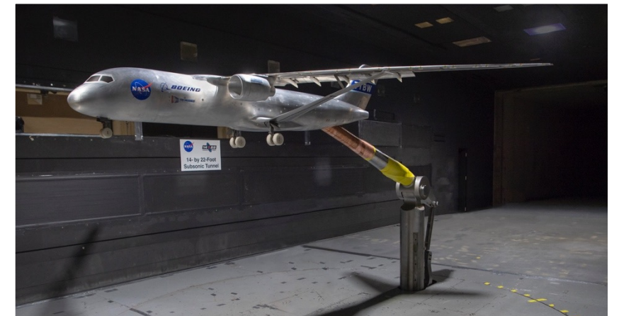
NASA/Boeing 8% Scale Low-Speed Performance Test NASA Langley 14- by 22-Foot Subsonic Tunnel
