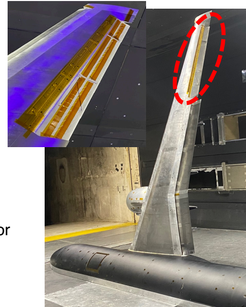
CRM-HL Test of AFC on Aileron in 14x22 Tunnel, 2023
