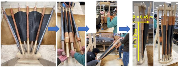
Fig. 8. Folding steps of the first gore MDU using a wood fixture consisting of seven push rods (four on the outside and three on the inside of the gore) that generate three lobes in the shell. The outside rods are hinged at the bottom to enable 90° upwards rotation.
