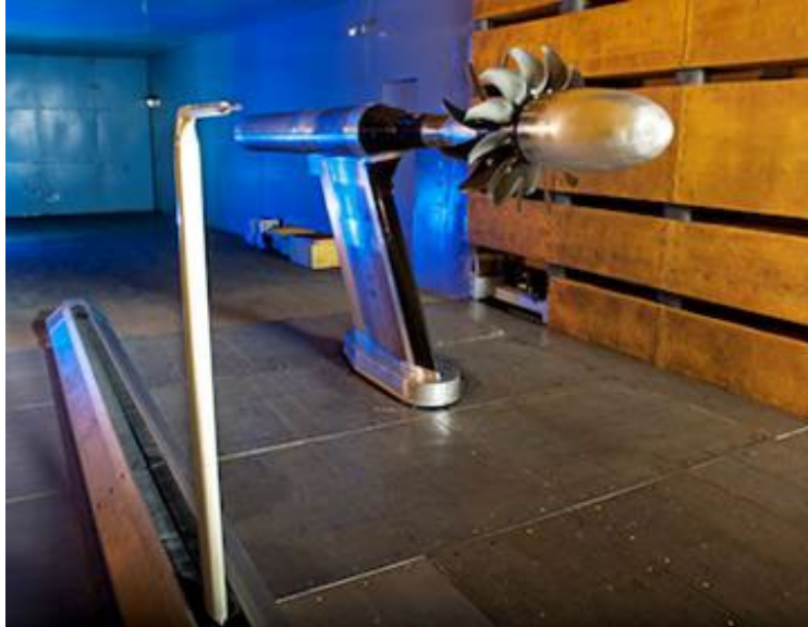
Open rotor with pylon (RDG 359)
