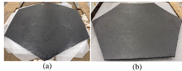
Fig. 12. 1-m-wide hexagonal panel cores fabricated. (a) Backside of the side panel; (b) reflective side of the central panel.
