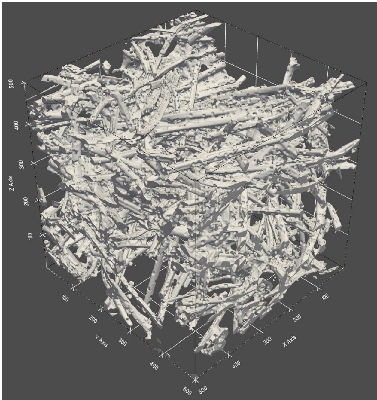
Figure 1: FiberForm sample with oxidative etch pits obtained from SPARTA and used within PuMA to compute various material properties.
