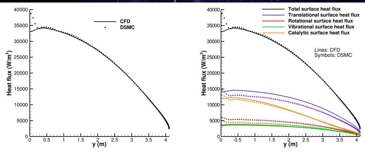
Excellent agreement in total heat flux, despite discrepancies in each separate heat flux contribution from the various modes.
