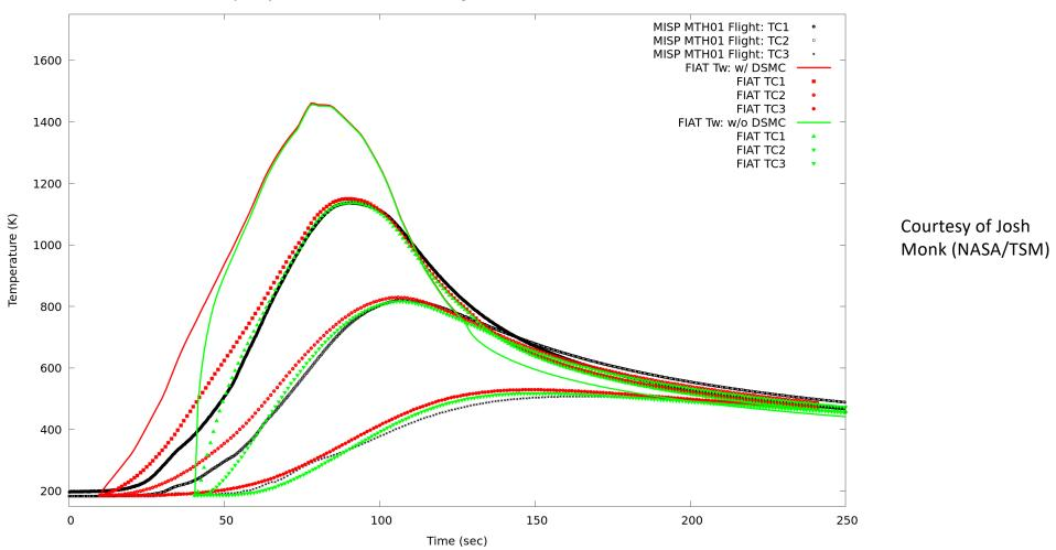
While the additional heat load between EI and 35 s is small, it is obvious that neglecting contributions from early time points entirely affects the surface and in-depth temperature response for a long time.
