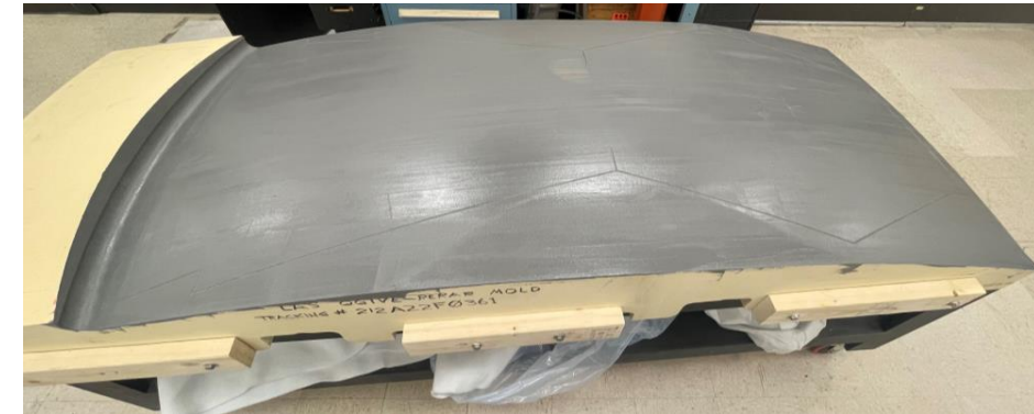
Fabricated 30° gore mold with SPIDER paraboloid
