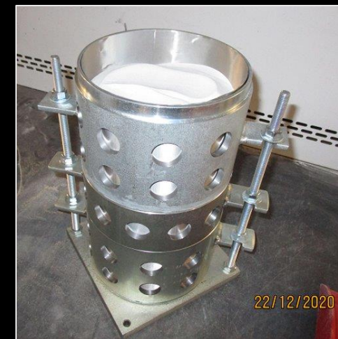
Vented Prototype Regolith Bin Design (NASA KSC)
