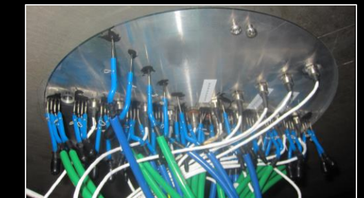
Instrumented Impingement Plate (NASA LaRC/MSFC)
