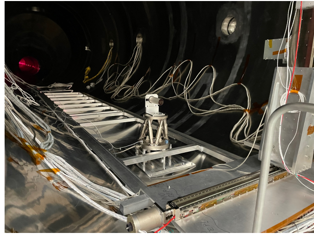
Figure 4. SSAXI mounted mirror module on the facility's hexapod. The Parker Stage, with the facility's CCD camera and focal plane SDD, positions detectors in the focal plane. The red laser light is used to facilitate coarse alignment and focusing the test article.
