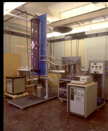
Falling-Film Heating/Evaporation Facility
