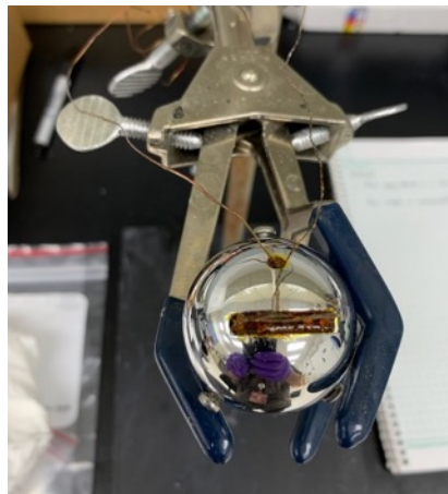
Figure 10 – Photo of highly polished aluminum sphere with the superconductor temperature sensor installed.
