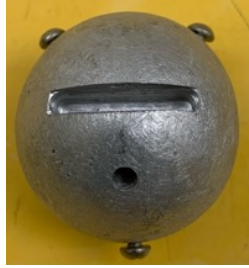
Figure 1: 37.4mm diameter aluminum sphere (ADC12/A383) with pocket for the HTS and the silicon diode temperature sensor. The stainless-steel screws are for mounting and suspending the sphere in the deep space simulator.
