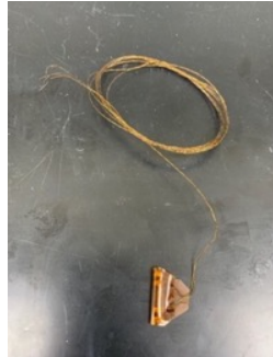
Figure 2: BSCCO 2223 HTS sample with 36-gauge wire attached for a four-point resistance measurement to monitor the superconductor transition. The HTS has been wrapped in Kapton tape to prevent electrical contact with the aluminum sphere.
