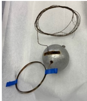
Figure 3: Aluminum sphere with the HTS sample and the silicon diode temperature sensor inserted and secured with a low temperature varnish.
