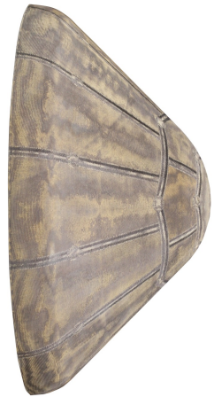
3D TPS woven with carbon and phenolic fibers infused with an ablative resin
