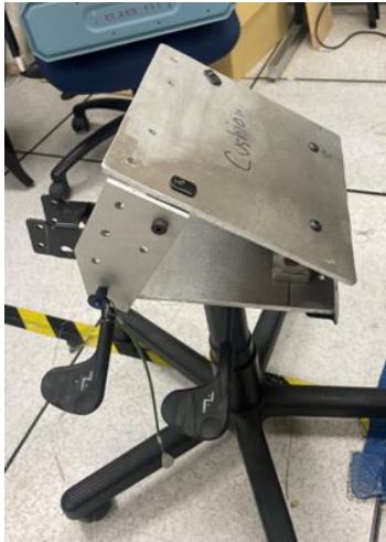
Figure 40. Final Design of Tilting Mechanism Bolted to Shock and Base Structure of Chair
