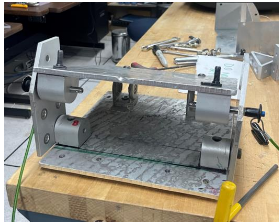
Figure 38. Final Design of Tilting Mechanism for Seat Pan: Rear View
