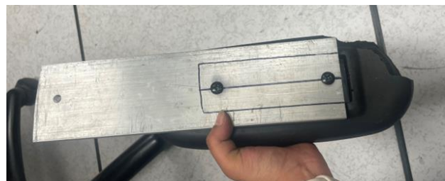
Figure 31. Aluminum Plate Bolted to Base of Armrest
