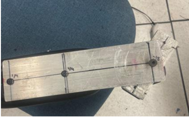
Figure 32. Aluminum Plates Connected with Shoulder Bolt
