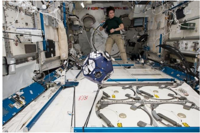
Figure 5. ISS Handrails on Floor and Walls
