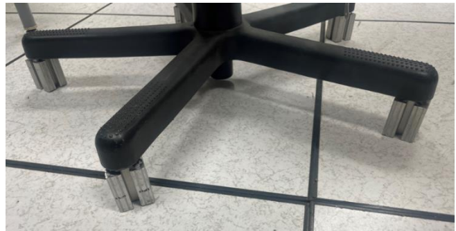
Figure 35. 80/20 Blocks Replacing Wheels on Chair Base
