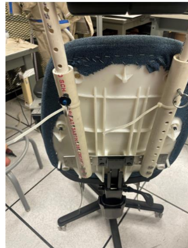
Figure 26. Seat back with Telescoping PVC Pipe Fixtures
