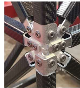
Joint under loading
