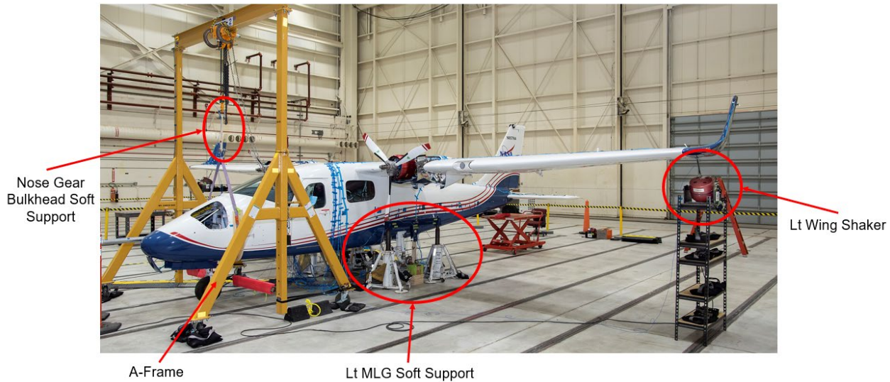
Figure 1: Previously conducted X-57 Mod II Aircraft GVT setup on soft supports to simulate a free-free boundary condition.
