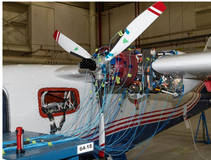
Figure 2: X-57 Mod II Cruise Motor GVT setup performed with aircraft on its landing gear.
