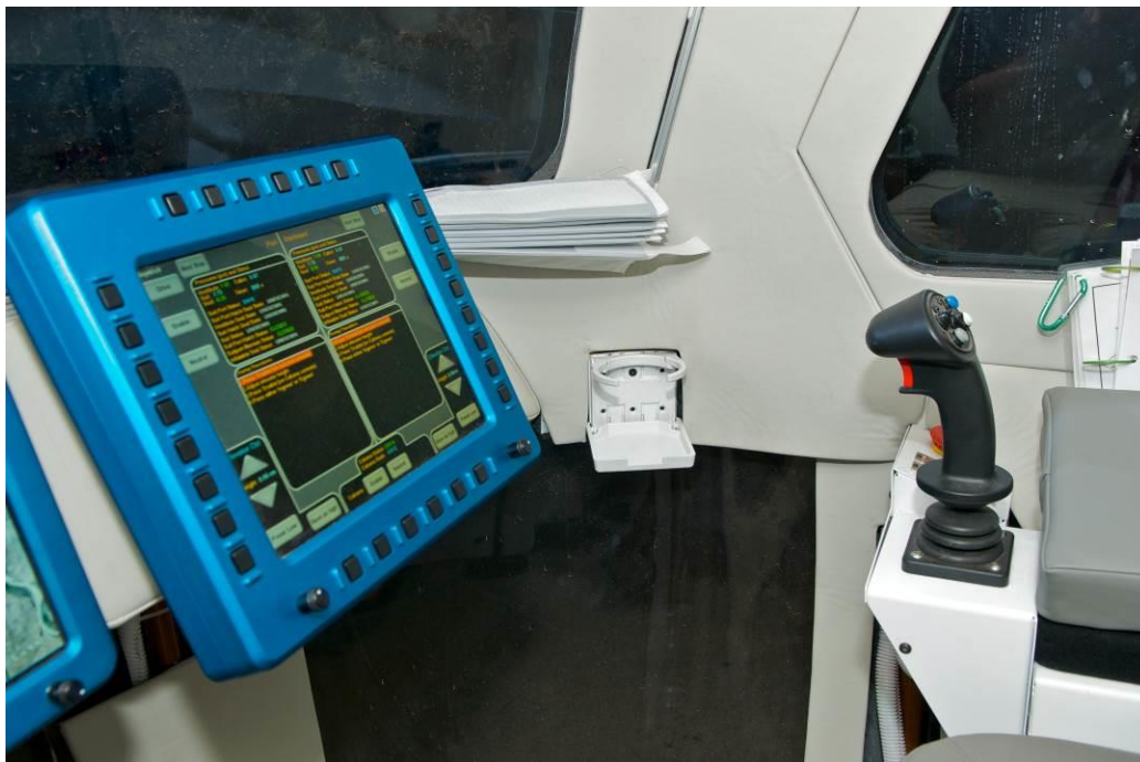
Figure 23. The CH Product MV4 Joystick in the SPR Generation 1B cockpit during field testing in 2009.
