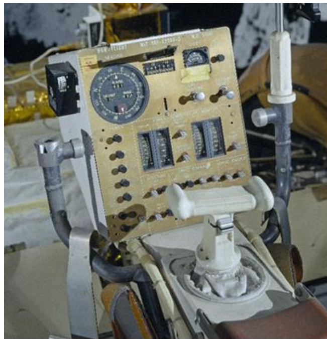
Figure 22. The Apollo LRV T-Handle controller and center display console. [Curiosity NASA]
