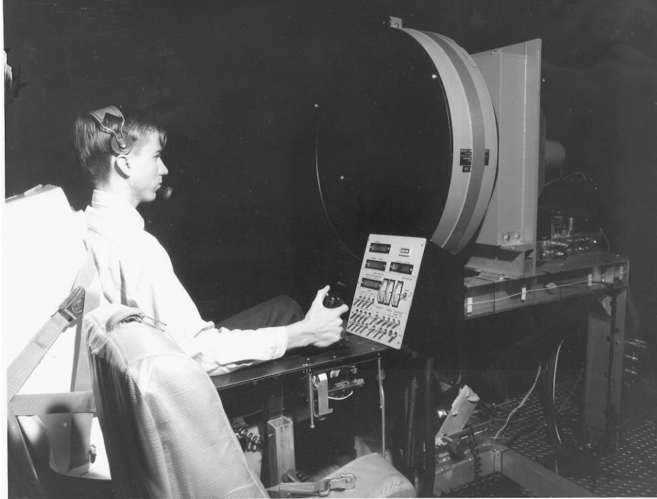
Figure 3. A subject using an Apollo type vertical pistol grip controller in an LRV simulator with a large circular TV monitor display [5].
