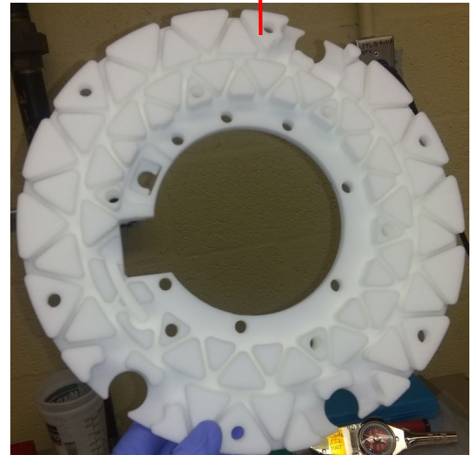
Sample Internal Foam Insulation (~11" diameter)
