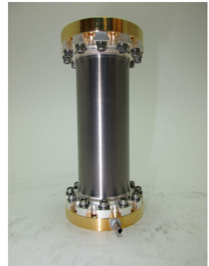
Active Gas Gap Heat Switch – as-built
