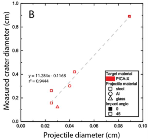
Figure 7B: Cross-plot of PICA-X damage feature size and projectile diameter
