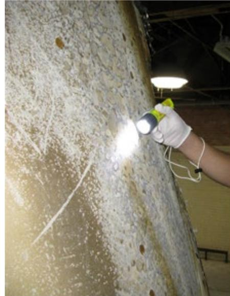
Figure 2B: MMOD post flight inspection initial screening technique
