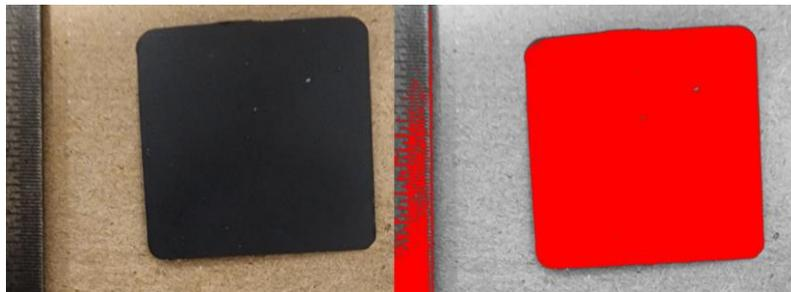
Fig 2. ImageJ analysis of pristine Kapton® XC sample used to estimate area for erosion yield calculations
