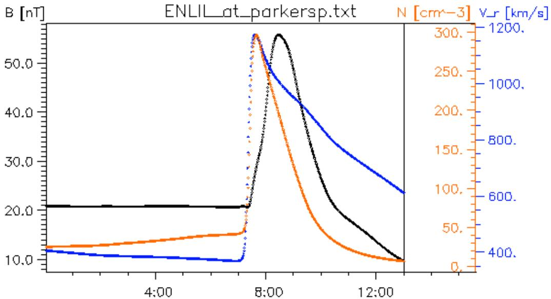
**Figure 9.** Magnetic field strength (black), plasma number density (red), and radial component of the solar wind speed (red) as a function of UT, DOY 47, 2022 from the ENLIL model of the 16 Feb 2022 CME at PSP.
