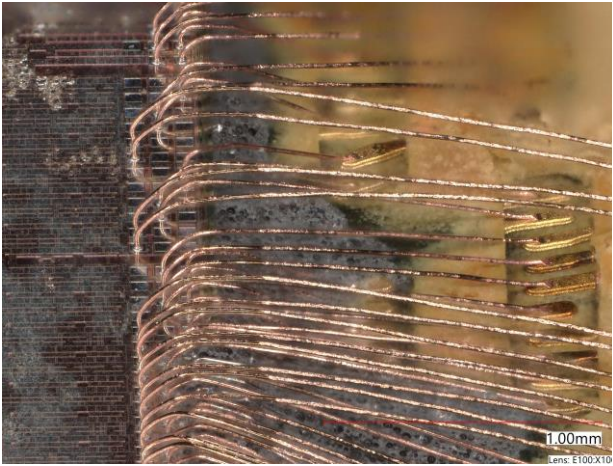
Figure C.3-10. Representative Optical Image of Multi-Tier Component (M7-MCK-LFBGA169-01).
