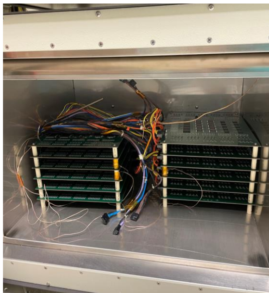
Figure B.7-7. Temperature Cycling Test Set-Up of Boards in Oven
