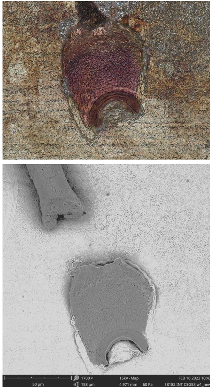
Figure C.3-20. Representative Optical and SEM Images of M5-MCK-VSSOP8-01 Showing Wire That Broke with Low Force Following Decapsulation and Bond Pull in Post-1000 TC Condition
