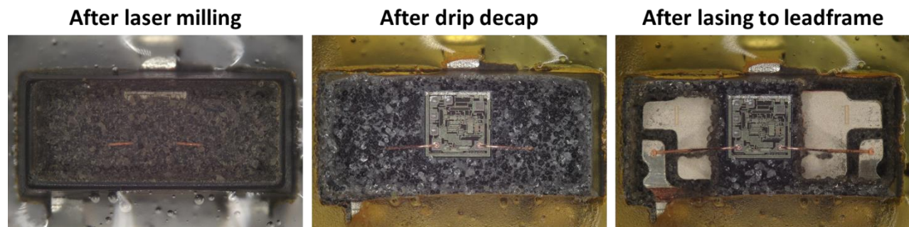
Figure C.2-3. Images Representing Stages of Decapsulation Involving Drip Decapsulation
