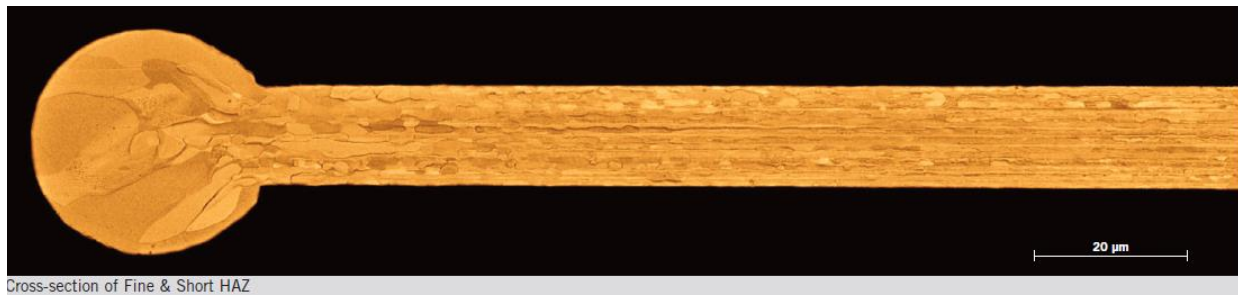
Figure A.1-17. Micrograph of 2N Au Wire Cross-Section, Showing FAB, HAZ, and Wire Grain Structure
