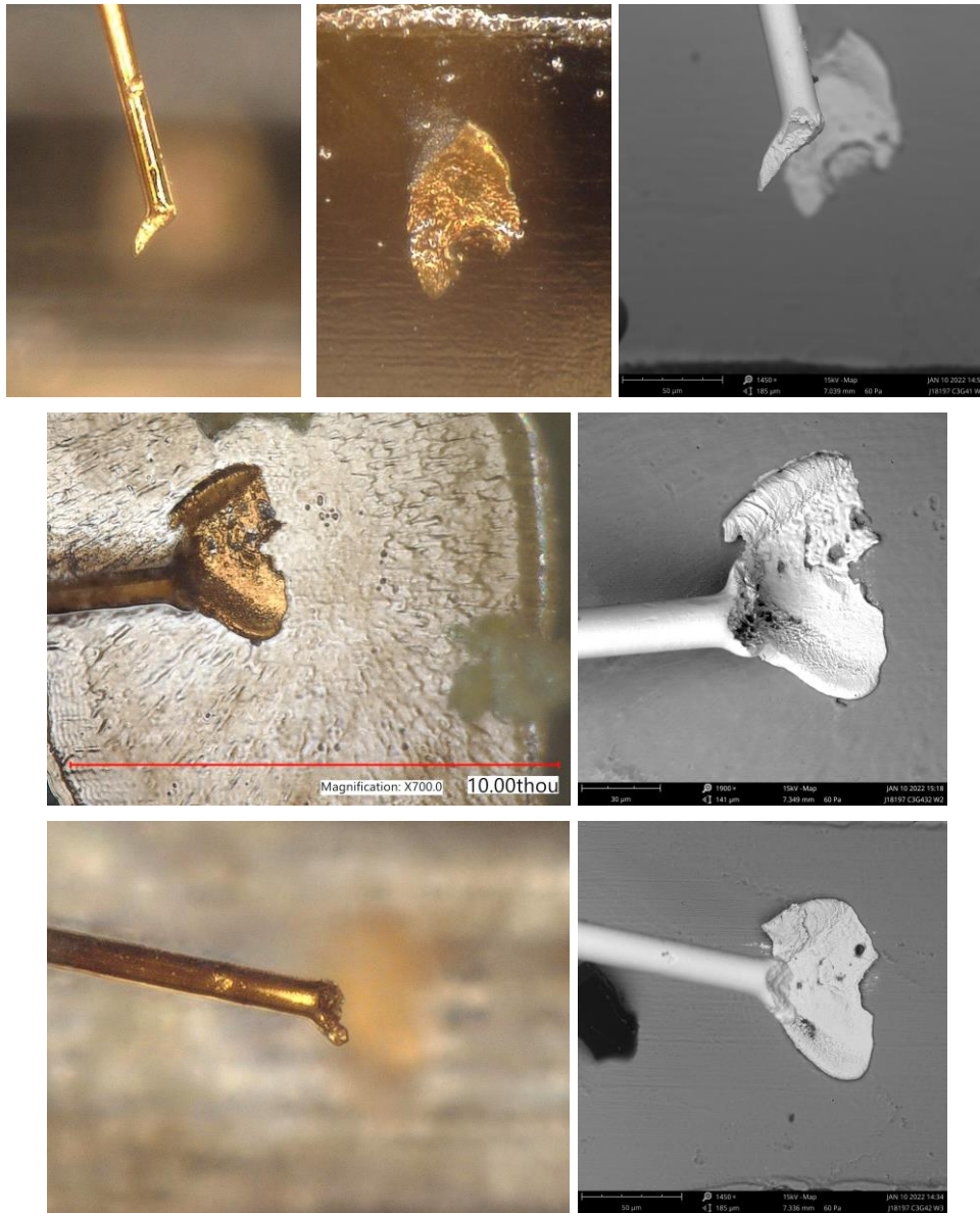
Figure C.3-14. Optical and SEM Images of Stitch Bond Wires That Broke at Low Forces Following Decapsulation and Bond Pull of M5-MCK-SOT235-01 (Au) in post-2000 TC Condition
