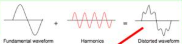
Fig. 1-6 Conceptual diagram of harmonics waveform. http://www.iea-pvps-task10.org/IMG/pdf/rep10_06.pdf
