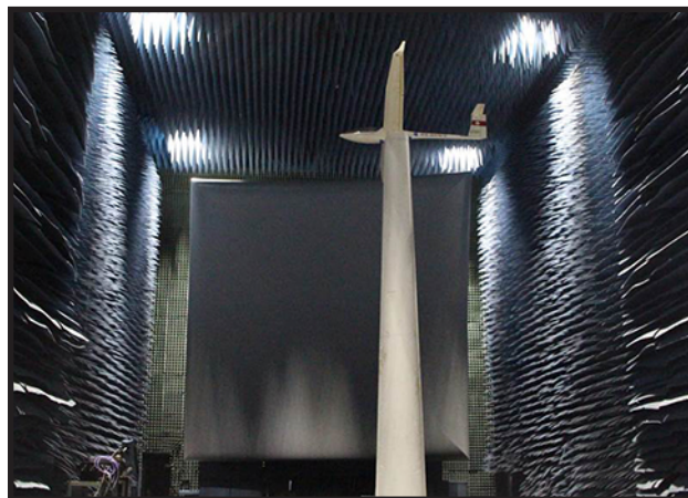
EM characterization of drone, shown mounted on foam column in ETR.
