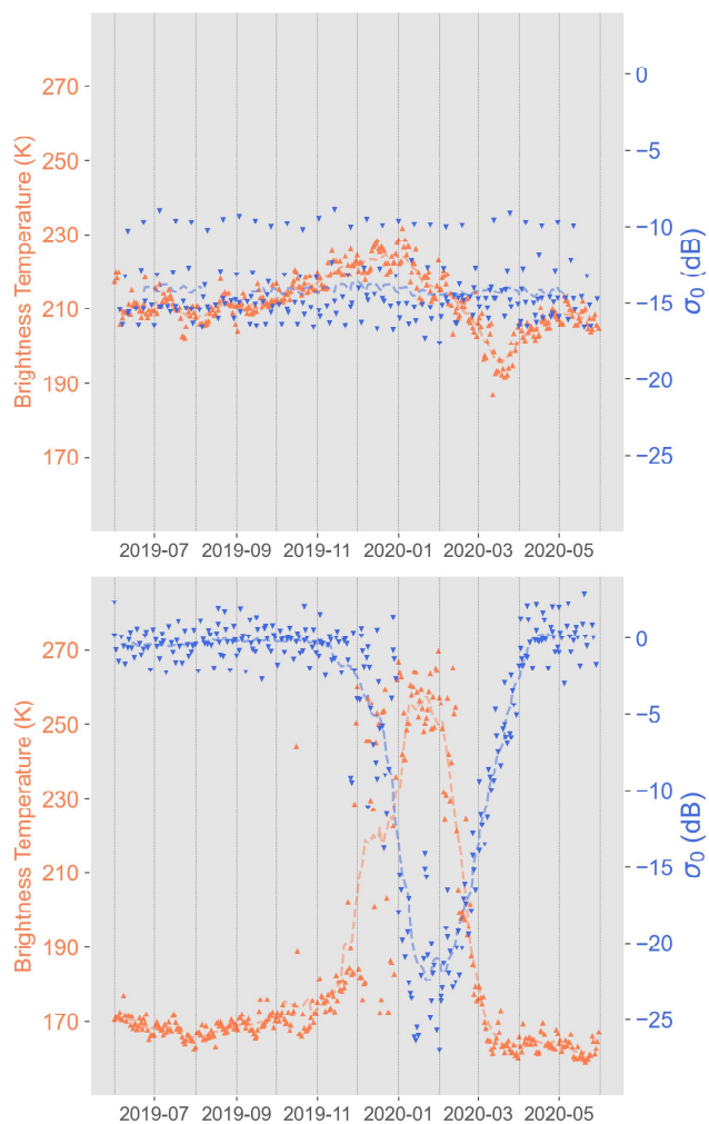
Figure S 1. Evolution of backscattering coefficient \sigma_0 (in blue) and brightness temperature (orange) over the Larsen C ice shelf (top, 67.54°S 63.90°W) and the Wilkins coast (bottom, 68.08°S 65.86°W) over the 2019-2020 melt season. In a place where no melting is observed (top), \sigma_0 and the brightness temperature show almost no changes. On the contrary, in areas subject to melt (bottom), we can observe a decrease of \sigma_0 and an increase in the observed brightness temperature.
