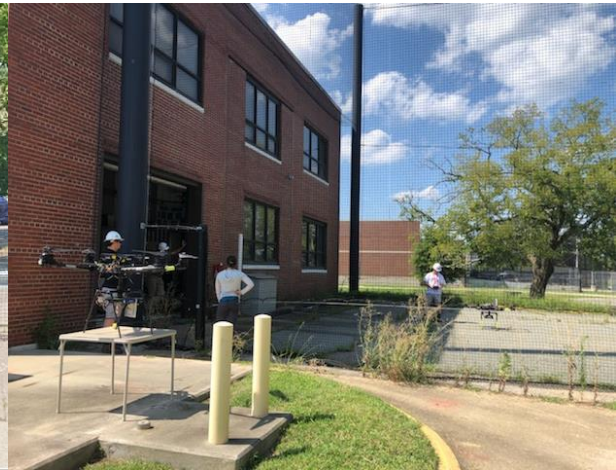
Figure 17: Cage testing of Ad-Hawk payload on board an Alta X
