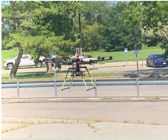
Figure 16: Cage-testing of NEST payload on board an Alta 8
