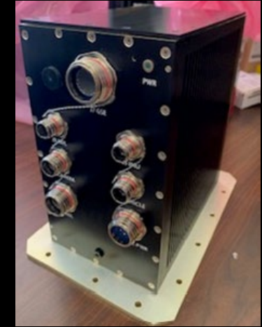
Safe and Precise Landing – Integrated Experiment (SPLICE) Descent and Landing Computer (DLC)
