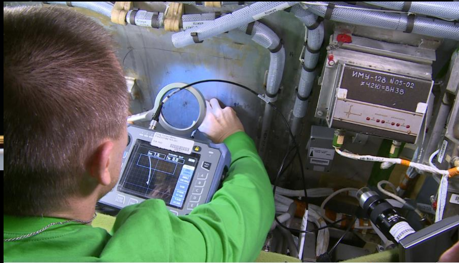
Eddy Current for crack sizing
