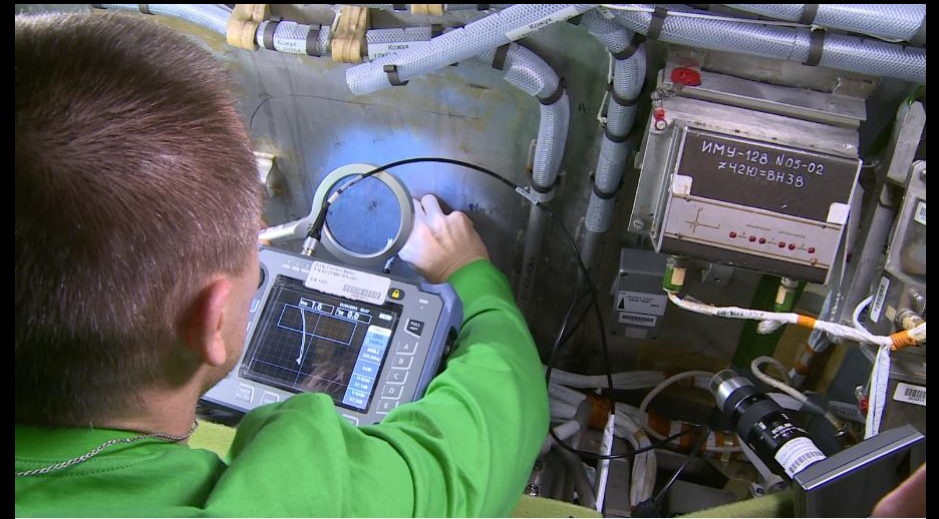
Using a Nortec 600D Eddy Current system on-orbit
