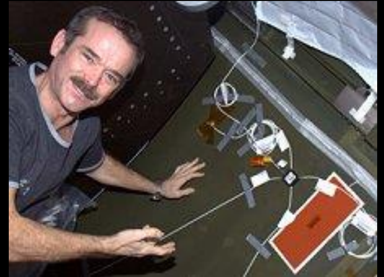
Canadian Space Agency astronaut Chris Hadfield, Expedition 34 Flight Engineer, installing SHM sensors behind a rack in the Destiny laboratory of the International Space Station.
