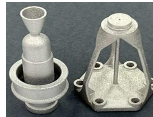
AM C103 Green Propulsion Thruster and Stand-Off.
