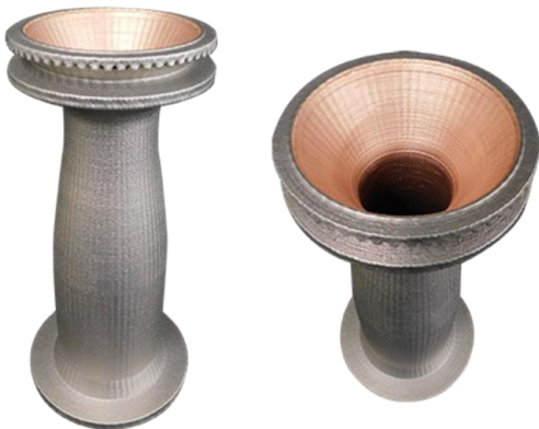
LP-DED Bimetallic Combustion Chamber
