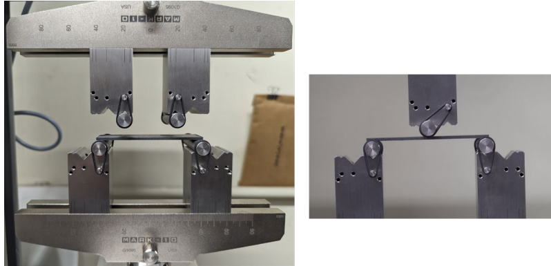
Fig. 3. Photograph of bending test rig in the original 4-point bend configuration (left), and the 3-point bend configuration (right).
