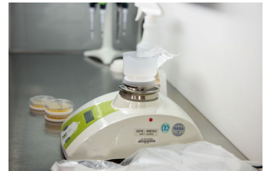
Membrane filtration setup.
