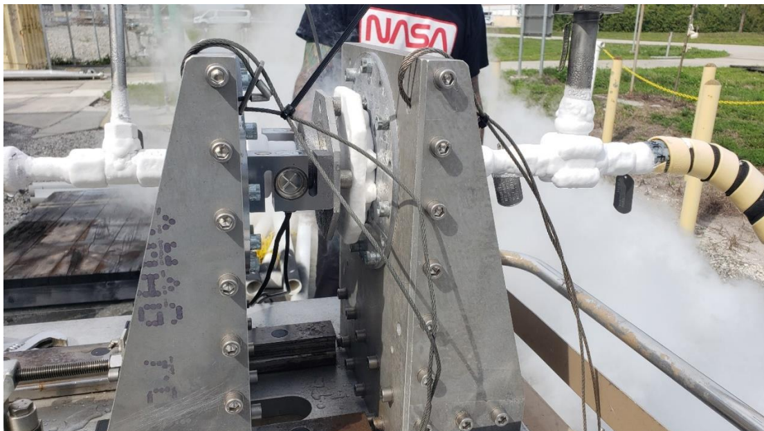
Fig. 29 Ice formation during the cryoflow test at the Kennedy Space Center.
