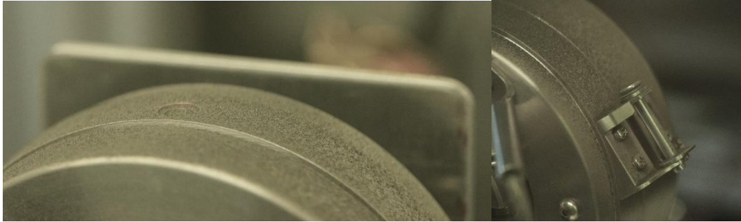
Fig. 23 Closeup of dust application on the CryoMag Coupler during testing in the UDDS chamber.
