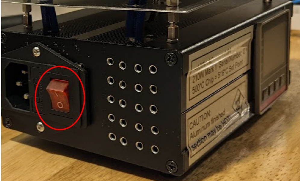
Figure 2.—Back panel of black (electronics) project box. Note power switch orientation.
