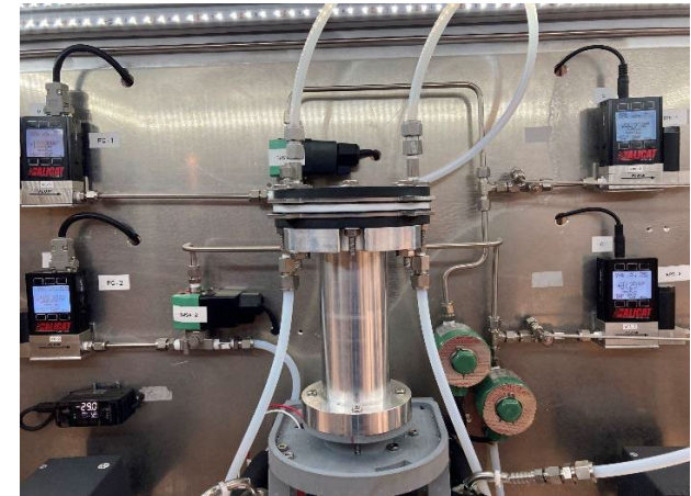
MFECR installed into the Electrolysis Test Stand
