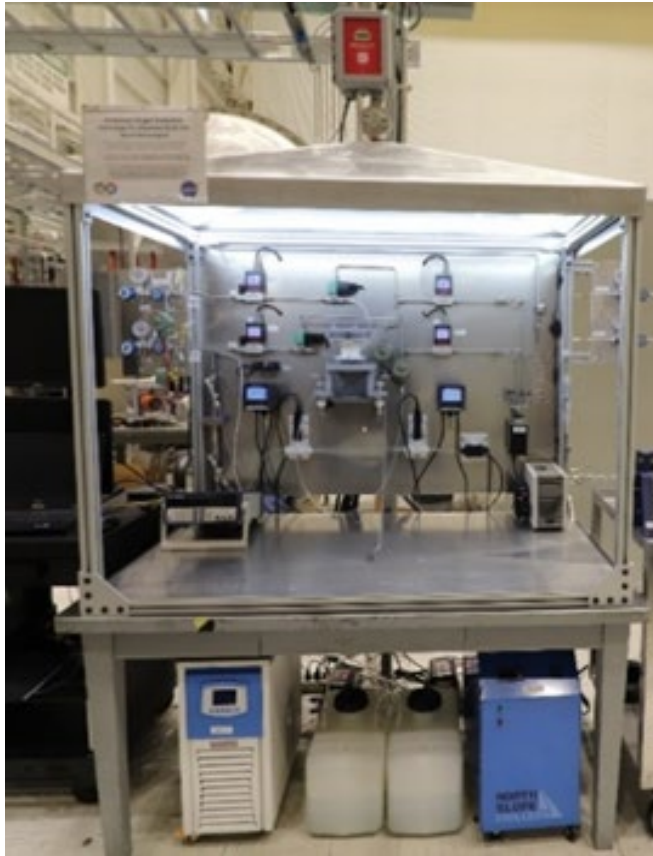
Electrolysis Test Stand
