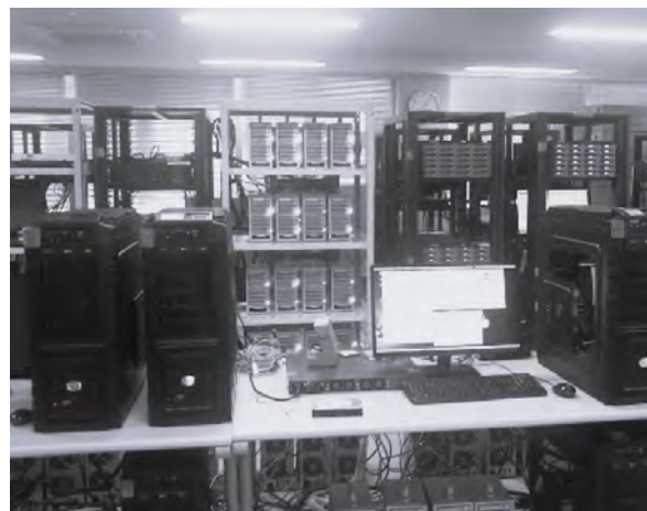
Fig. 1 View of the Mizusawa Software Correlator and data servers in Mizusawa Correlation Office.
