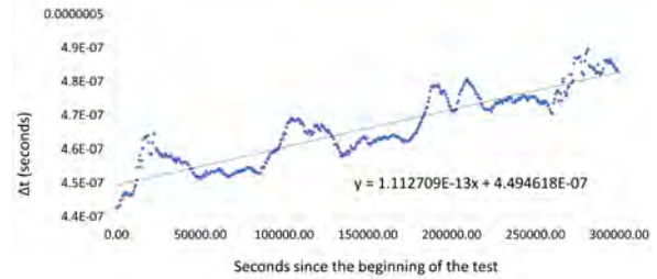
Fig. 6 Time difference between GPS and Maser PPS signal during 84 hours in December 2022.
