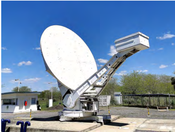
Fig. 2 The 6-m primary focus offset radio telescope for VLBI observations of AGGO (2021-10-16).
