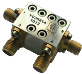
Fig. 5 30 dB cryogenic directional coupler.
