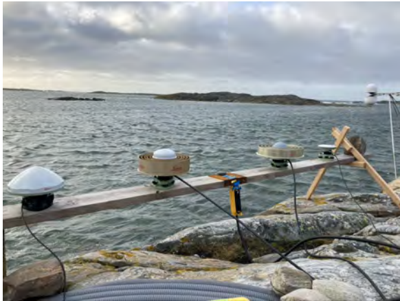
Fig. 1 Several different GNSS antenna types mounted close to the sea next to the permanent GNSS-R installation at Onsala (right).
