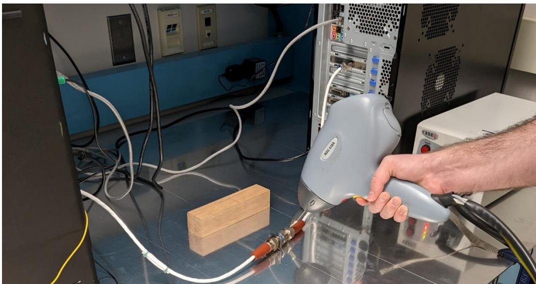
Figure 6.8-4. Application of Static Discharge using ESD Gun to Network Connector No data packet errors were detected when the connector was placed in electrical contact with the aluminum ground plane that was connected to Earth ground.
