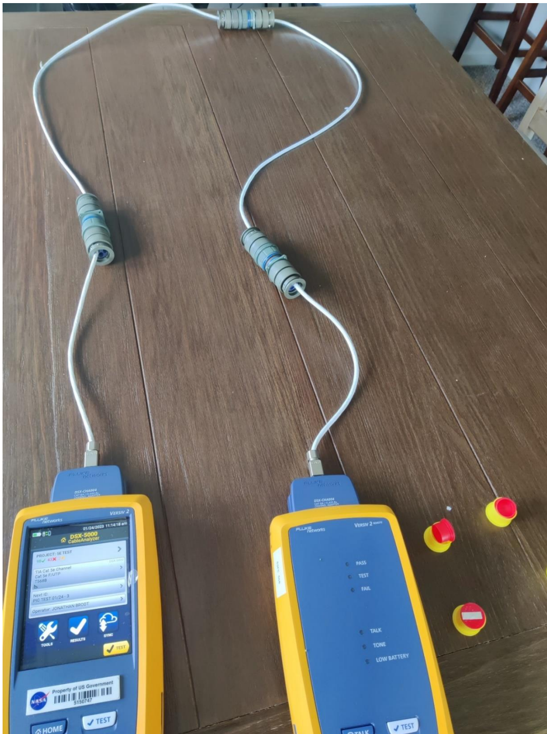
Figure B-64. Cable Analyzer Setup with PIC Connectors showing Three 1-m Segments connected through Four PIC Connectors
