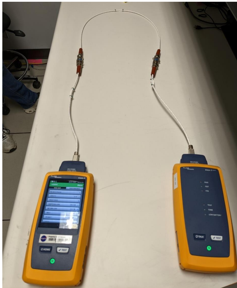
Figure 6.6-1. One Ethernet Cable Segment with Two CeeLok FAS-X Connectors in Series with Adaptor Cables Connected to Fluke DSX-5000 Meter
