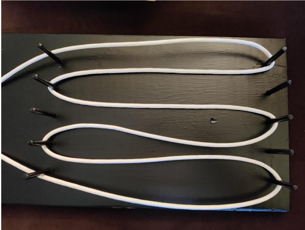
Figure B-91. Gore Ethernet Cable in Bend Fixture with Three Severe Bends (one times (1x) the cable diameter), Each with a Bend Radius much less than 4x Cable Diameter Requirement for Ethernet Cable
