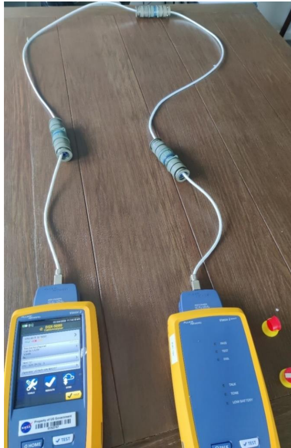
Figure 6.6-12. Cable Analyzer Setup with PIC Connectors showing Two 1-m (39.4-inch) Segments Connected through Three PIC Connectors
