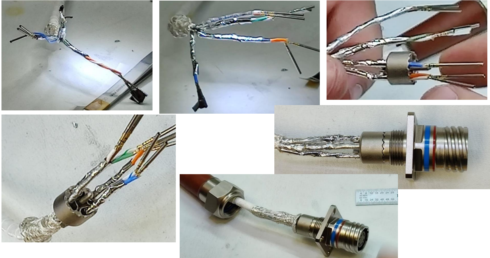
Figure 6.6-5. Detailed Second Re-termination Process (Ethernet cable re-termination that maintained wire pair twist and shielding added to each connector, resulting in passing cable analyzer Cat6a test using five cable segments and six connectors) Note each twisted pair is shielded so that shield is as close as possible to the connector grommet (less than 0.125 inch) when the contacts are inserted into the connector.
