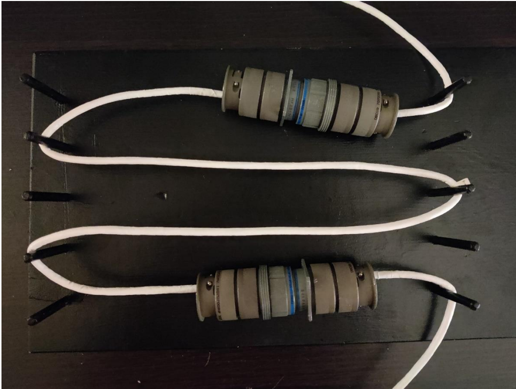
Figure B-95. PIC Ethernet Cable with PIC Connectors in Bend Fixture with Three Severe Bends (1x the cable diameter) each with a Bend Radius much less than the 4x Cable Diameter Requirement for Ethernet Cable
