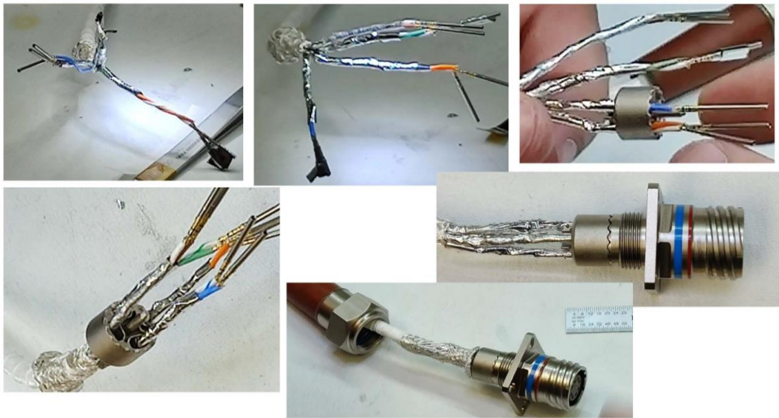
Figure A-1. Photo Documentation of Ethernet Cable Retermination that maintained Wire Pair Twist and added Shielding to Each Connector, Resulting in Passing the Cable Analyzer Cat6 Test using Five Cable Segments and Six Connectors
