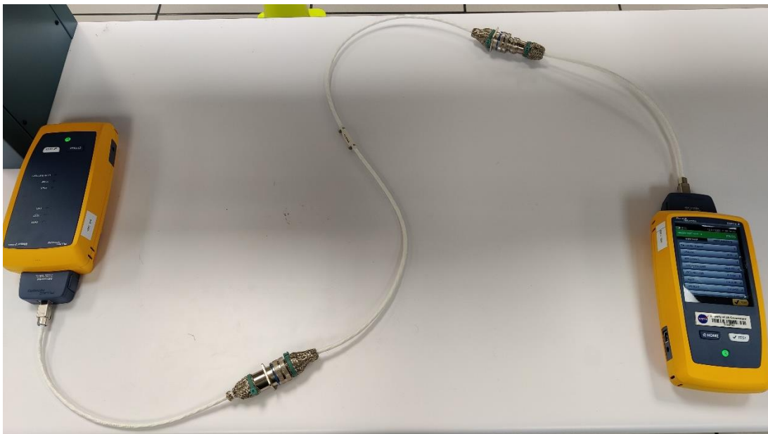
Figure 6.5-2. Fluke DSX-5000 Connected to RJ45 Adaptor Cable and 1-m (39.4-inch) Ethernet Cable Terminated with Ethernet Connectors Ethernet cable meter with transmitter is shown on the right, and the unit on the left reflects the transmitted data back to characterize the Ethernet cable.
