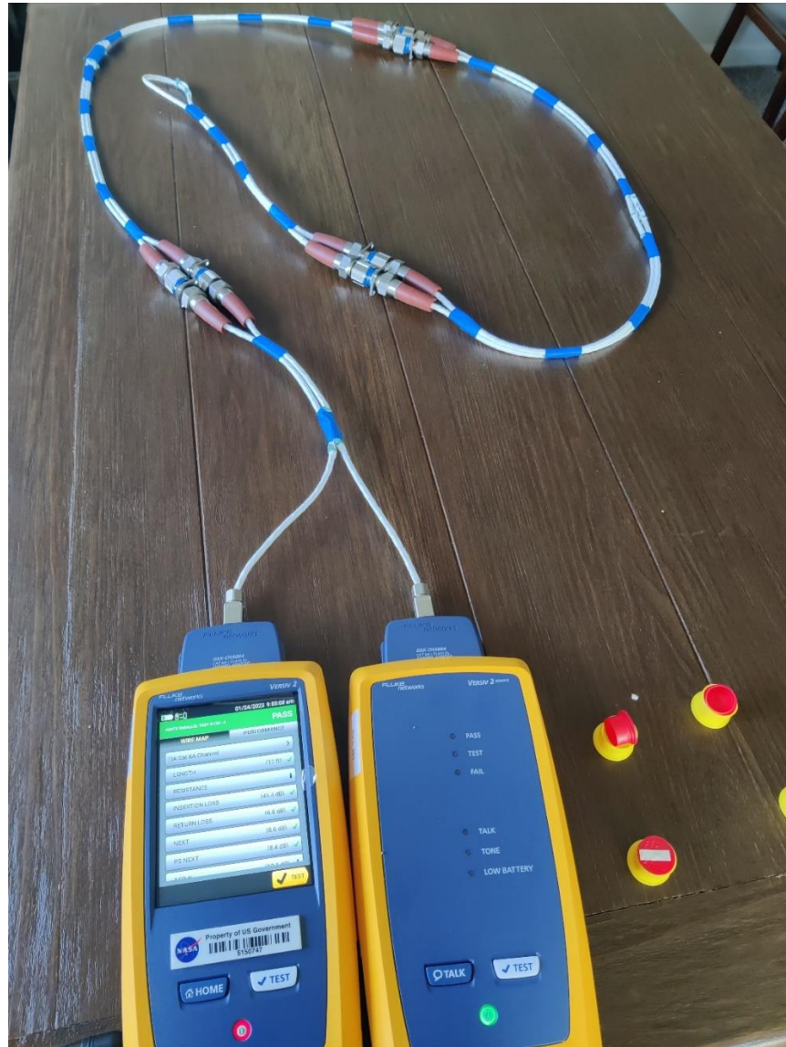
Figure B-79. Cable Analyzer Test with Five Gore Cable and CeeLok FAS-X Connector Segments adjacent to Measure Potential Crosstalk between Ethernet Pairs
