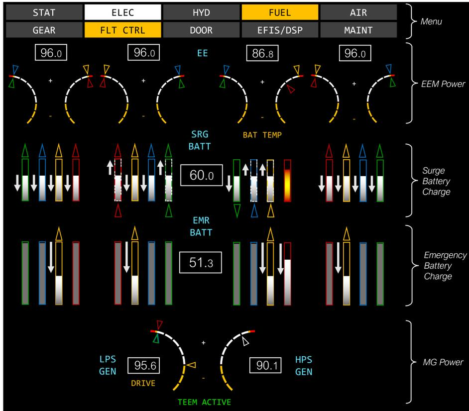
**Fig. 6 Laterally Arranged HESD.** In this example, the yellow LPS MG has failed, so the emergency batteries on the same bus are powering the yellow motors. Additionally, one of the red surge batteries has overheated. The tabs on the top row also indicate a warning in the fuel system page.
