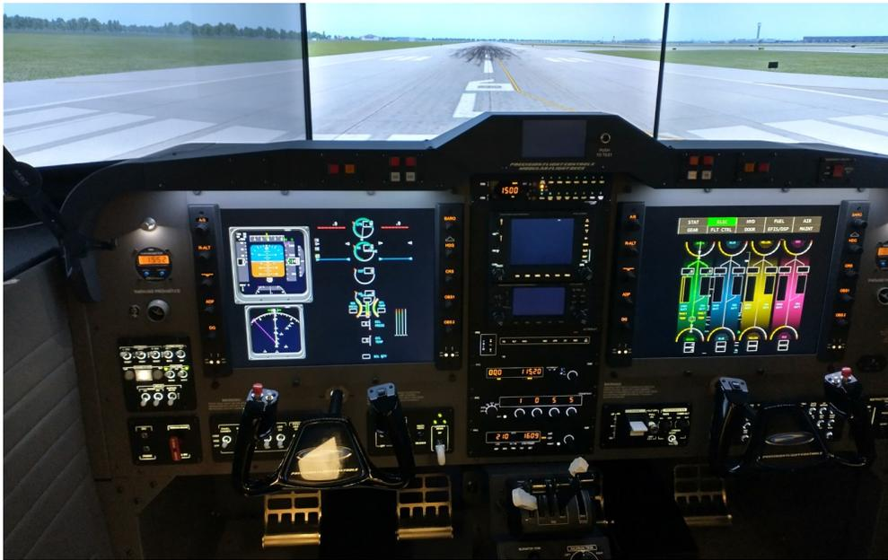
**Fig. 3** The flight simulator setup at GRC. An earlier iteration of SUSAN's EICAS and HESD is shown.
