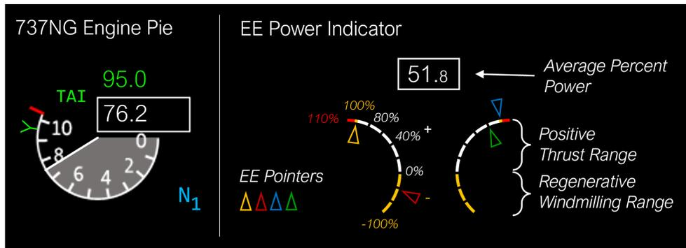
**Fig. 7 Engine pie used on the 737NG and Max [44] compared with the dial proposed for the HESD, which can display information about four separate EEs while occupying a similar width. *Italicized text are annotations.***
