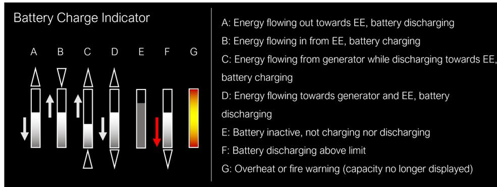
**Fig. 8** Examples of the battery charge indicator in different situations.
