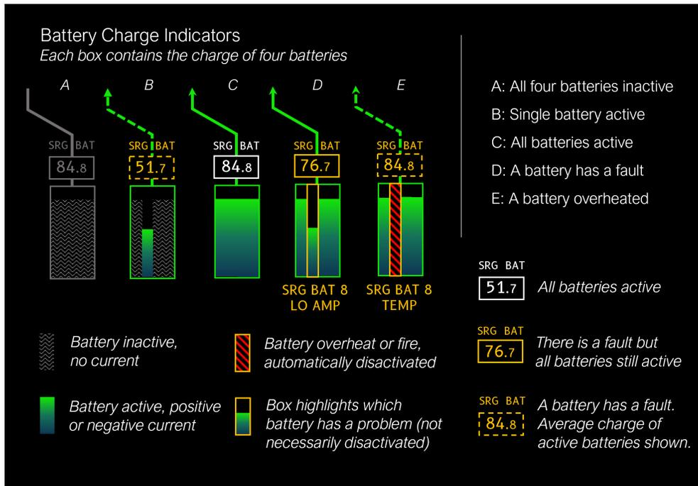
**Fig. 15** Examples of the battery charge indicator and its various warnings.
