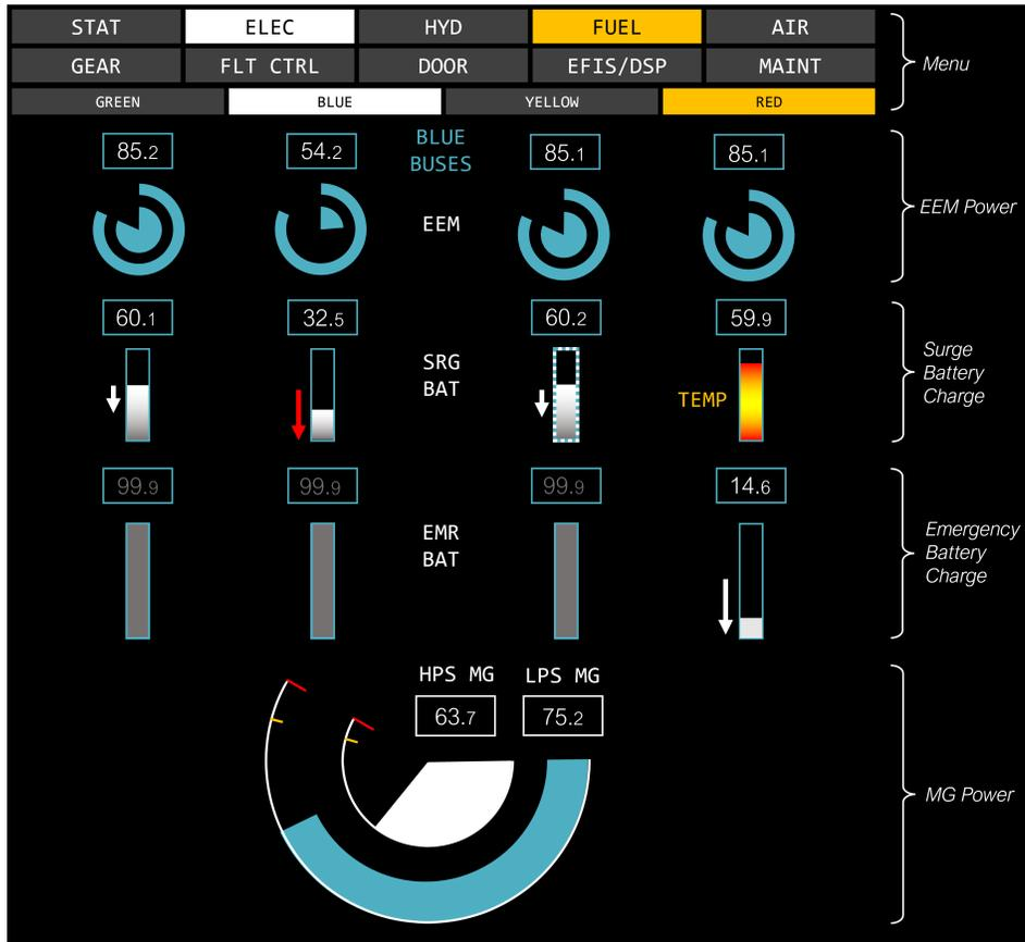
**Fig. 5** Example of a HESD concept displaying components connected to the blue LPS MG. The rightmost surge battery has overheated, triggering a temperature warning, and activating the emergency battery. The left inboard battery is also indicating an abnormally high discharge rate with a red discharge indicator.
