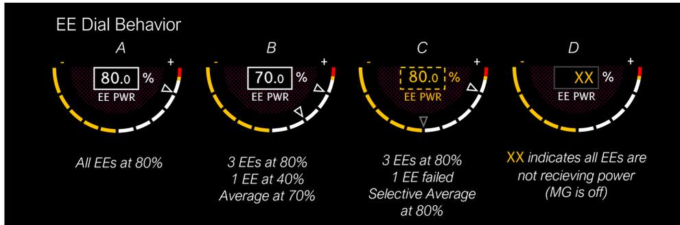
**Fig. 14** Various deviations between EE power shown on the EE dial. The MG dials work in the same fashion.
