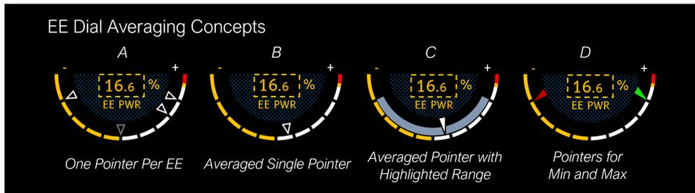
**Fig. 13** The four concepts explored for simplifying the EE dial. Digital readouts are in amber because one EE has failed.
