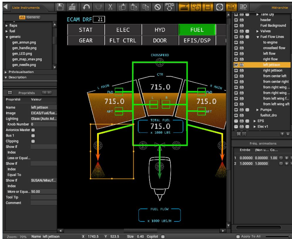
**Fig. 4** A concept fuel synoptic page for SUSAN inside Planemaker’s 2D panel builder.
