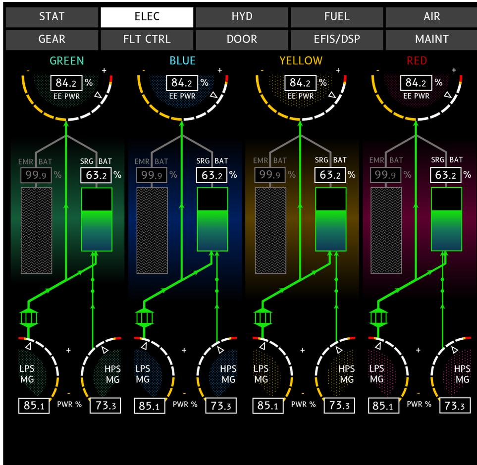
**Fig. 9** The Compartmentalized HESD under normal flight conditions. Instead of presenting 16 buses explicitly, the principle of compression gives the impression that there are only 4 main systems to monitor. The display features the recent B612 font developed by Airbus [54].
