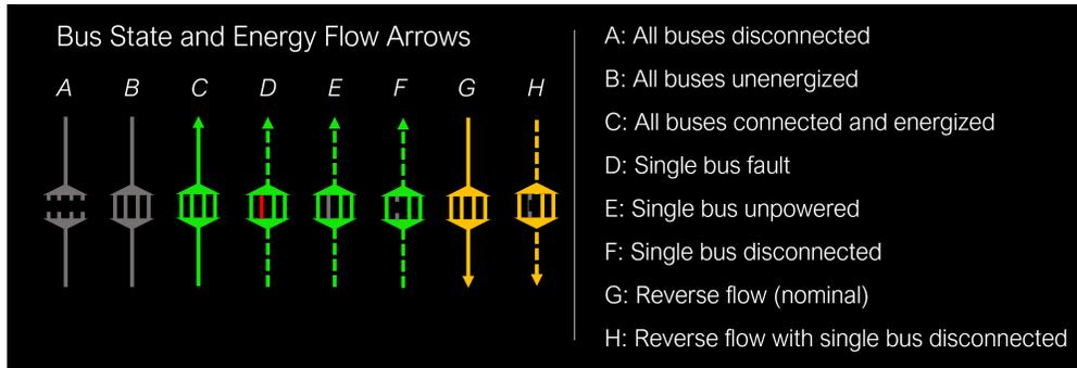
**Fig. 12** Examples of how the bus state indicator and energy flow arrow function.
