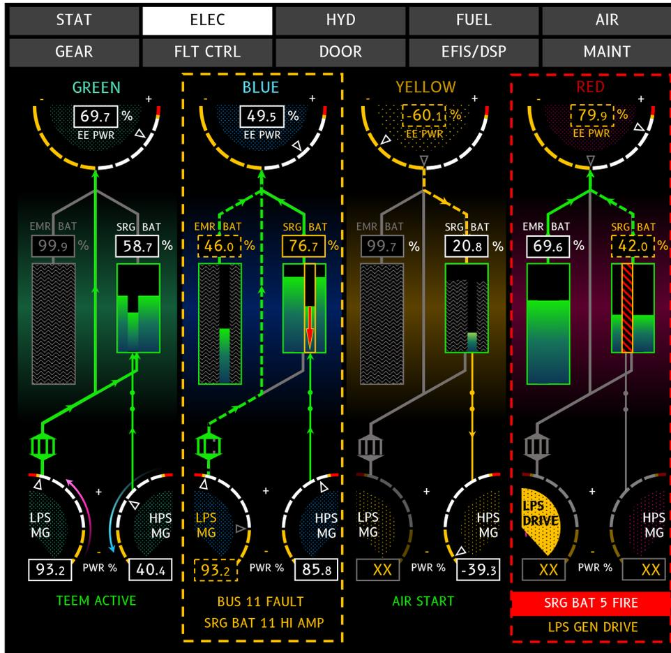
**Fig. 10 The Compartmentalized HESD in off-nominal operation. Each compartment depicts a different situation. The behavior of each individual bus is now visible.**
