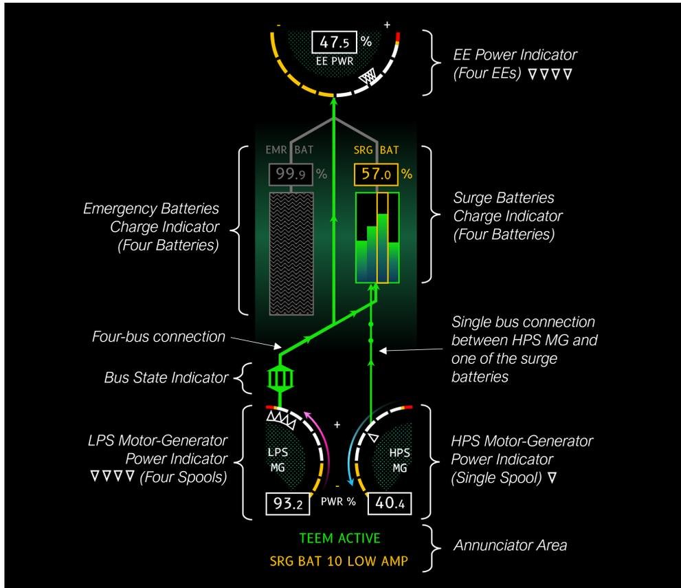
**Fig. 11 A single compartment of the display.**
