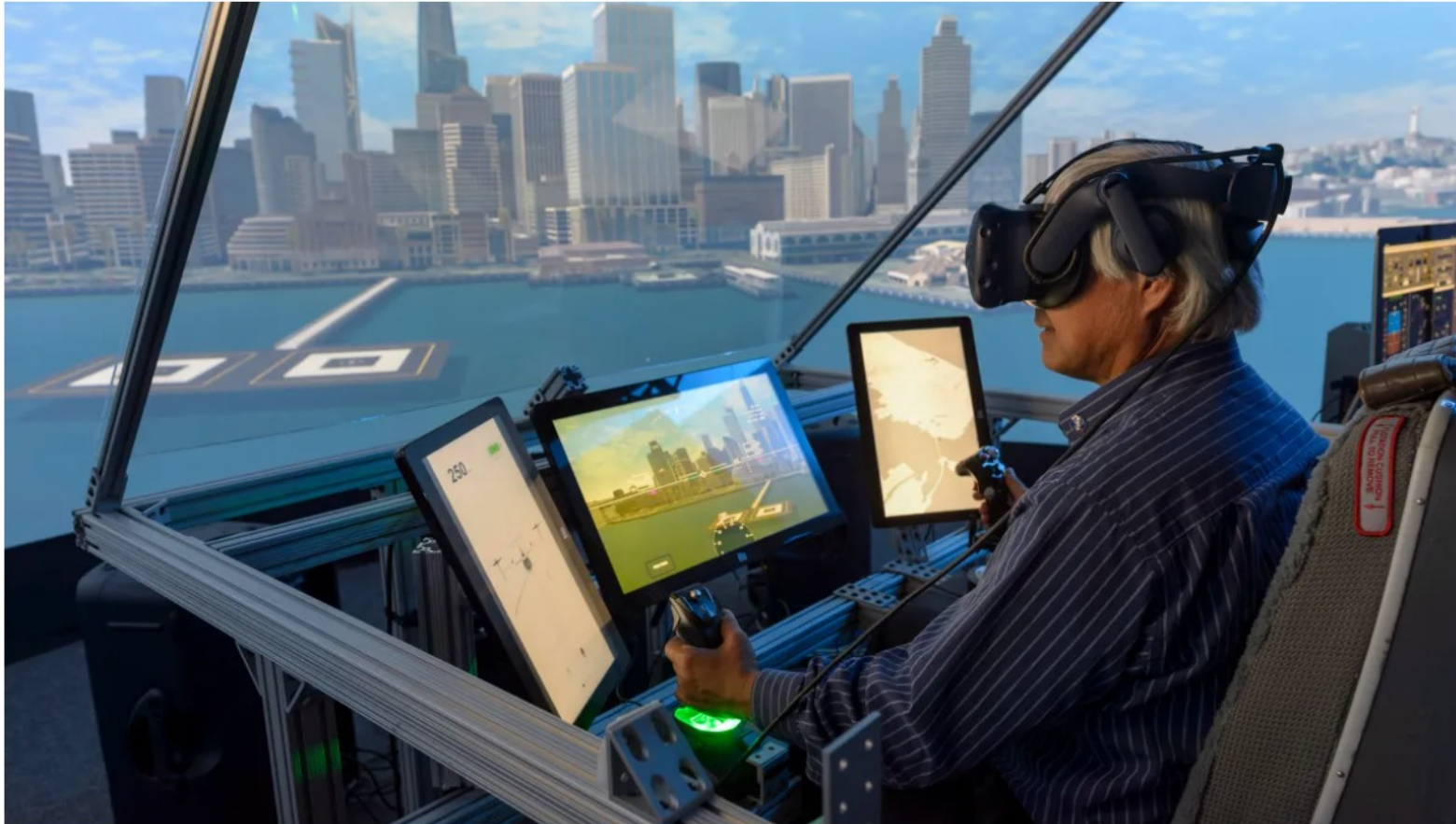
The Aerospace Cognitive Engineering Lab Rapid Automation Test Environment at Ames showing out-the-window views of San Francisco for an Advanced Air Mobility ride quality simulation project.
