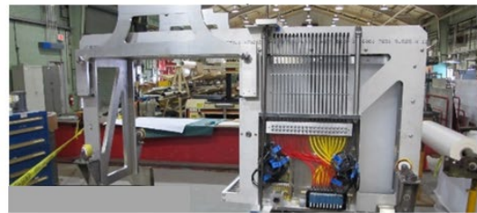
c) Polyethylene degrader system
