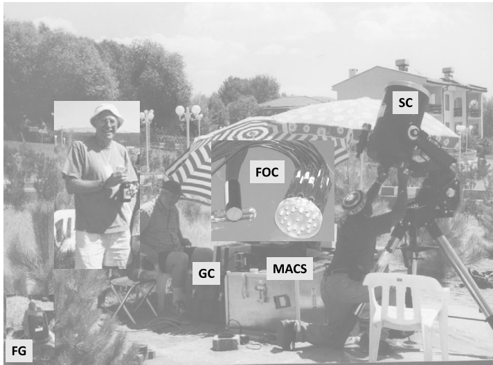
Figure 13 MACS experiment conducted during the total solar eclipse of 11 August 1999 in Elazig, Turkey. The NASA team comprised of Joseph Davila (seated), Nelson Reginald (kneeling), and Charles Condor (standing). Shown in the picture is the 12-inch Schmidt–Cassegrain (SC) telescope, spectrograph (MACS), ground computer (GC) to operate the camera, field generator (FG) for power, and the fiber optic coupler (FOC) with 21 fibers between SC and MACS. The image of the totality formed on the glass surface of the FOC and the slit face of the FOC illuminated the transmission grating in MACS. The totality lasted for 124 seconds.
