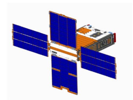
BioSentinel geometry analyzed by HZETRN2020. Top: fully detailed CAD model. Bottom: Combinatorial geometry.
