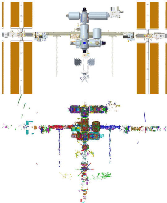
ISS geometry analyzed by HZETRN2020. Top: fully detailed CAD model. Bottom: Interpreted geometry from ray-trace information.
