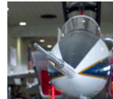
Shock sensing probe mounted on NASA F-15
