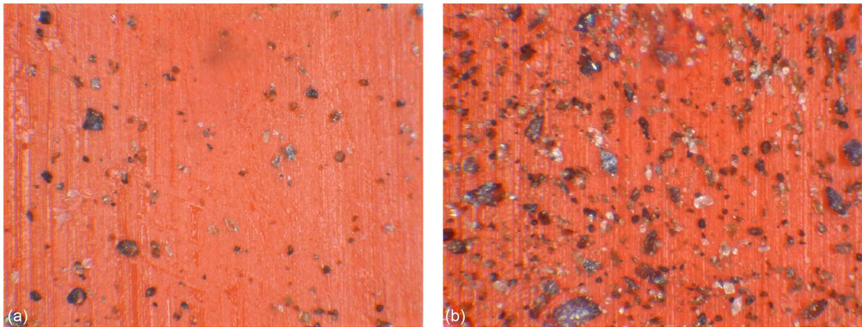
Figure 8.—Dust coverage on NDS seal test specimens. (a) Less than 14 percent. (b) Greater than 22 percent.
