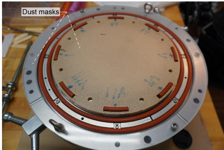
Figure 1.—NASA Docking System (NDS) seal in leak test fixture with dust masks installed.
