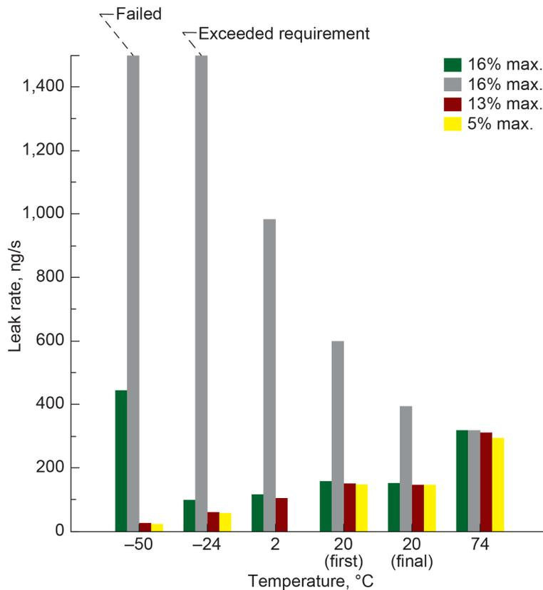
Figure 13.—Leak rates for subscale NDS seals with JSC-1A lunar simulant at various temperatures.
