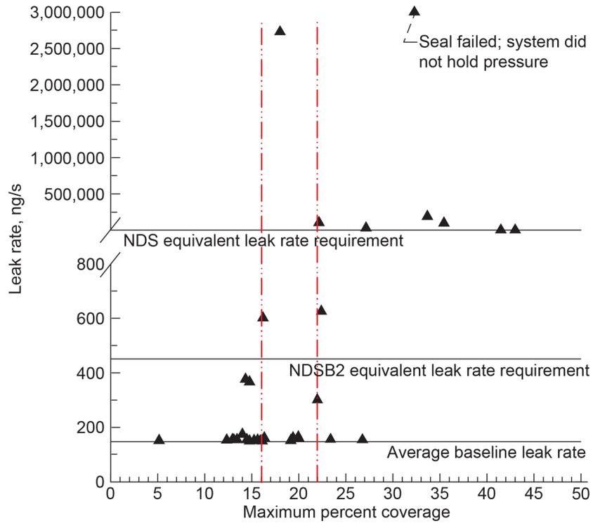
Figure 7.—Leak rates for subscale NDS seals with JSC-1A lunar simulant at 20 °C.
