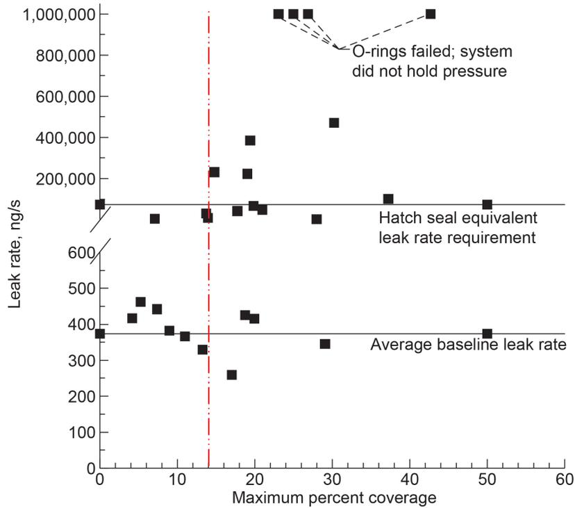
Figure 9.—Leak rates for subscale Orion docking hatch seals with JSC-1A lunar simulant at 20 °C.
