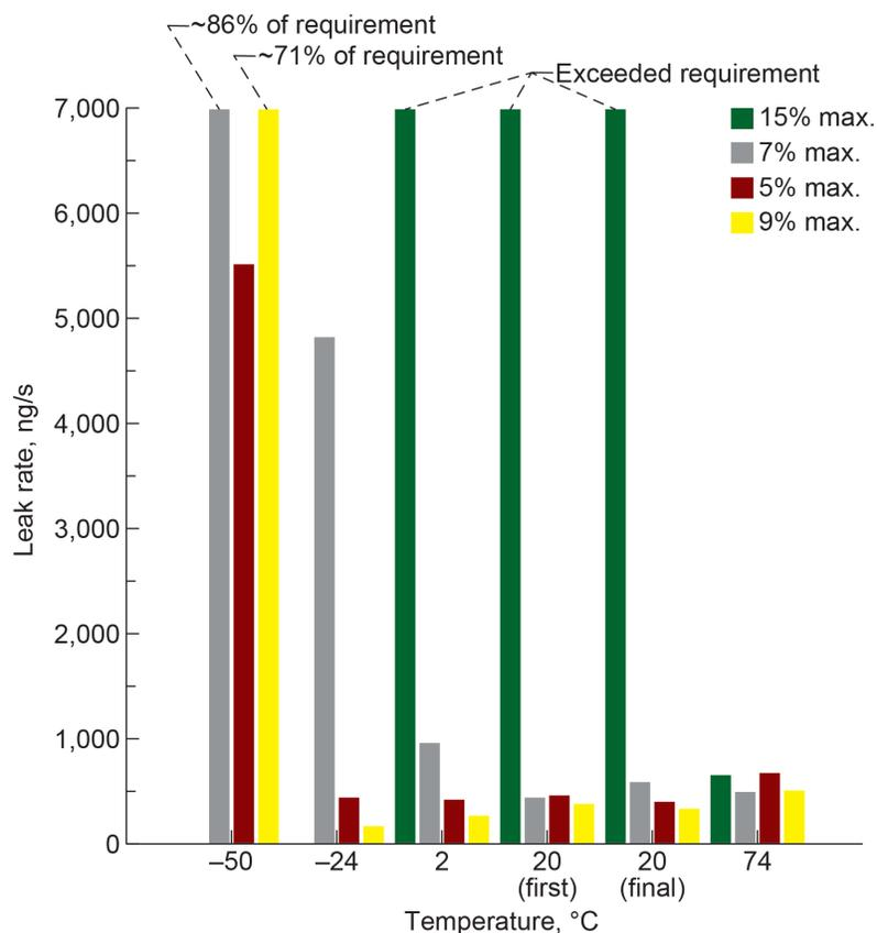
Figure 12.—Leak rates for subscale Orion docking hatch seals with JSC-1A lunar simulant at various temperatures.
