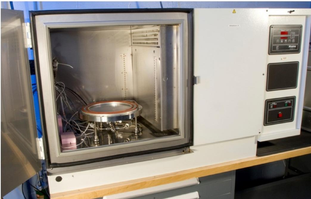
Figure 6.—Environmental chamber used for leak tests.
