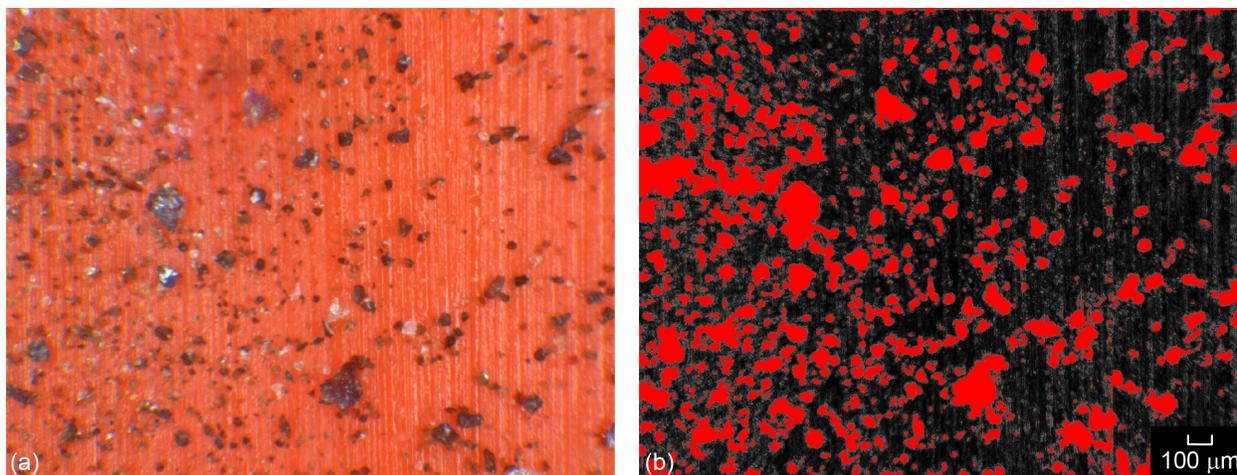
Figure 5.—Imaging output examples. (a) NDS seal with 22 percent dust coverage. (b) Segmented image using Fiji package.
