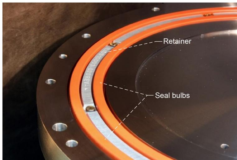
Figure 2.—NDS subscale seal installed in leak test fixture.
