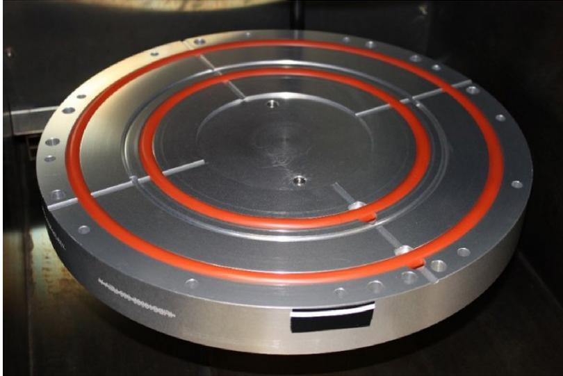
Figure 3.—Orion docking hatch subscale seal installed in leak test fixture.
