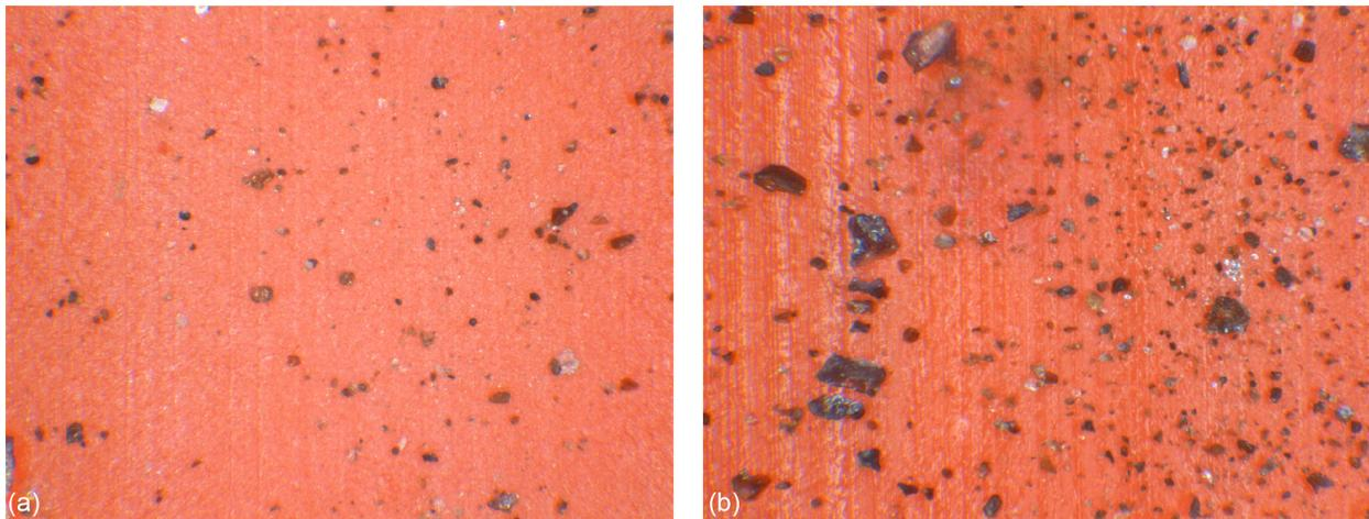
Figure 10.—Dust coverage on Orion docking hatch seal test specimens. (a) Less than 10 percent. (b) Greater than 14 percent.
