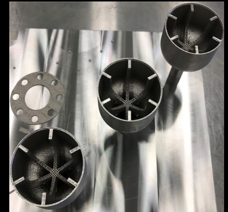
L-PBF AM IN718 integrated heat pipe funnels
