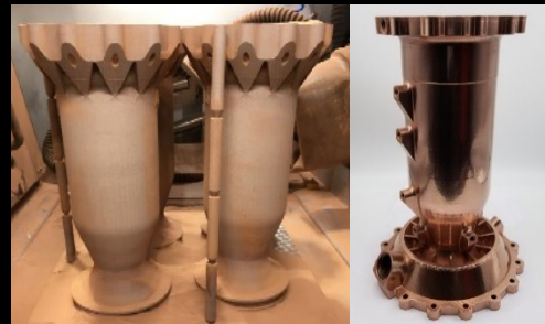
Laser Powder Bed Fusion (L-PBF) GRCop42. Courtesy Dr. Dave Ellis (NASA GRC).
