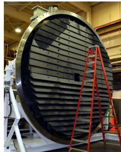
Fig. 3 Picture of the VF5 beam dump that the thruster fires into.
