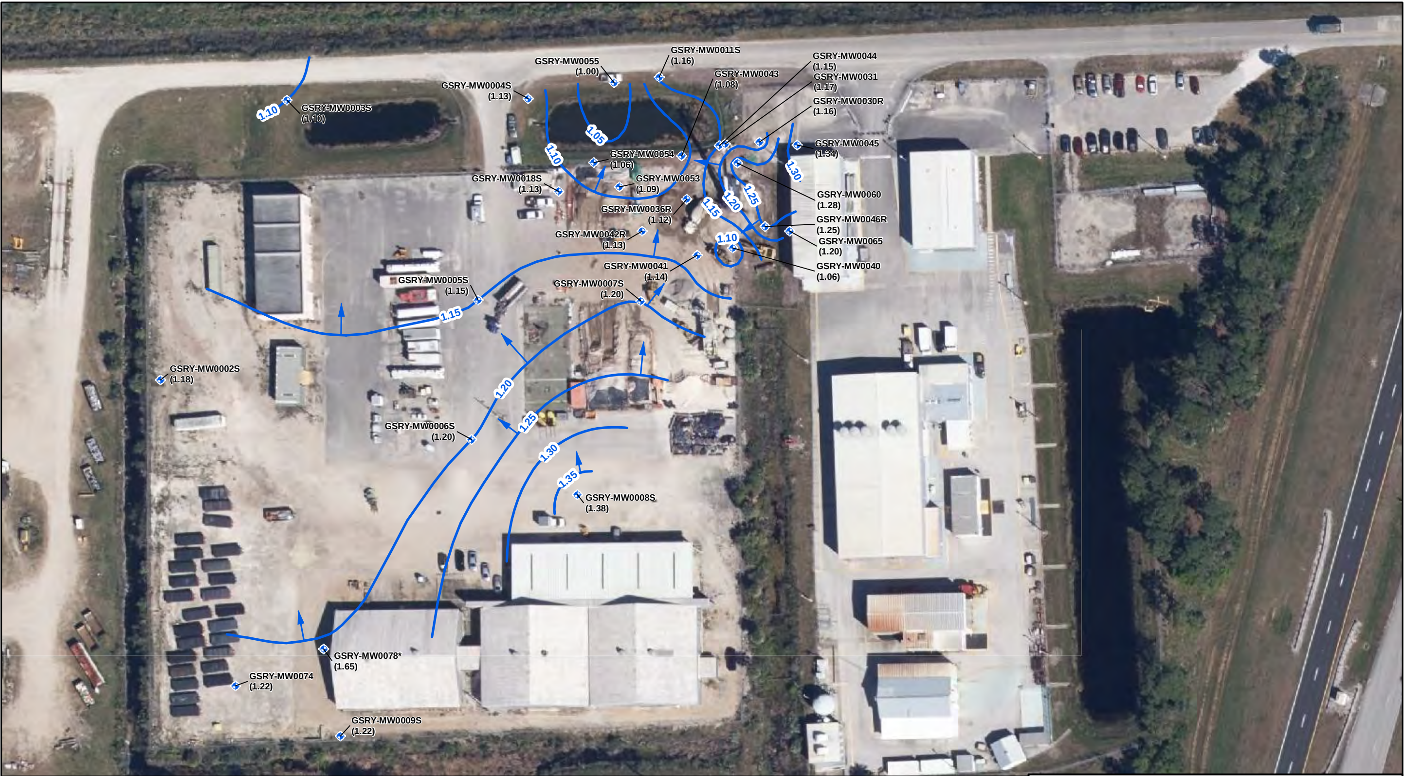
FIGURE 2-1 Groundwater Contour Map – September 27, 2022 2 to 18 feet bls General Services Administration Reclamation Yard (GSRY) SWMU 010 NASA Kennedy Space Center, Florida
