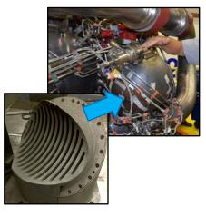
**RS-25 Pogo Accumulator Z-Baffle** Over 100 Welds Eliminated Nearly 35% Cost Reduction
