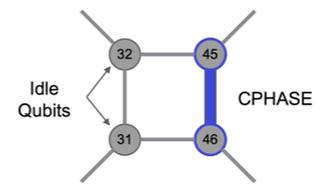
In a compiled circuit, Often when a pair of qubits undergo a two-qubit gate, to avoid degrading of gate fidelity the neighboring qubits are idle. This provides a natural time slot to apply DD without adding to the circuit length.
