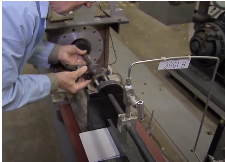
Fig. 6. Installing the guide tube assembly
