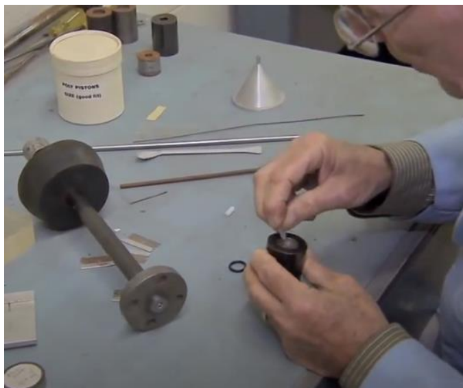
Fig. 4. Installing the diaphragm into the high pressure coupling
