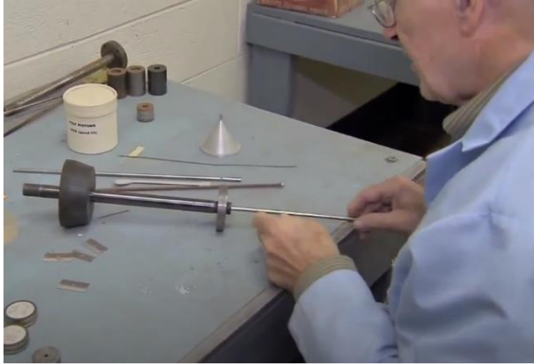
Fig. 5. Inserting the launch tube into the guide tube assembly
