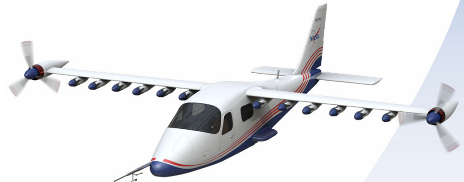
X-57 Mod IV in High-Speed (Cruise) Configuration
