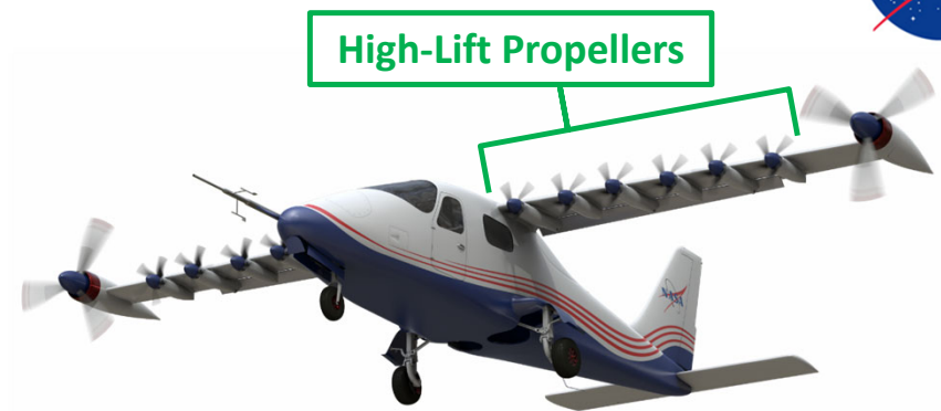
X-57 Mod IV in Low-Speed (Takeoff/Landing) Configuration
