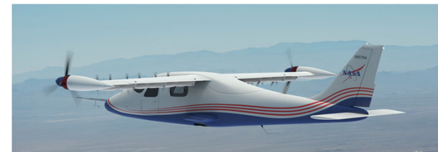
Mod III: Impact of cruise-sized wing, wingtip propellers
