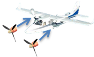
Mod II - Retrofit a Tecnam P2006T with an electric propulsion system
