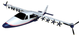
Mod IV - Design for low-speed takeoff and landing characteristics with an integrated Distributed Electric Propulsion (DEP) system.
