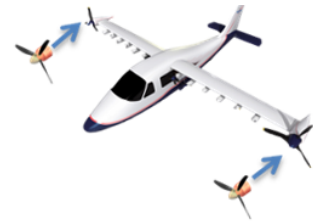
Mod III - Modify the configuration with a cruise-optimized wing and electric propulsion system
